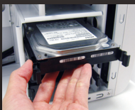
Installing a Hard Drive
